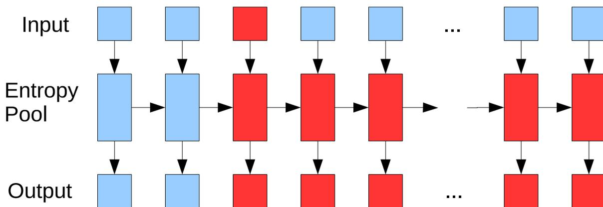
A 256-bit entropy pool is initialized with a well known value (256 zero bits). For each block of the
