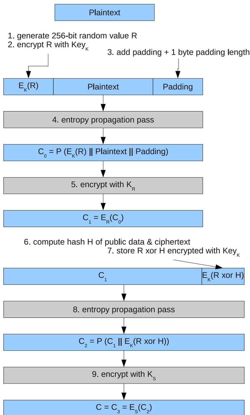
The hash H is computed like this: D shall be „the public data“ || 0xff, so if the public data is 0x20 0x20, D shall be 0x20 0x20 0xff. Then, D and C<sub>1</sub> are XORed together bitwise  $S = (D_0 \text{ xor } C_{10}, D_1 \text{ xor } C_{11}, D_2 \text{ xor } C_{12}, \dots)$ . The shorter of the two is padded with 0x00 bytes so that D and C<sub>1</sub> have the same length. Over this string S a SHA-256 hash is computed.
